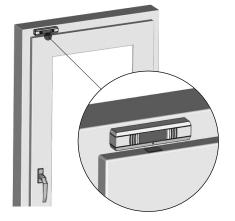
Mount the magnet flat as shown next to the arrow marking.
